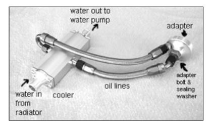
Installing this cooler is usually a simple task, depending on the chassis, radiator, and water hose routing. A look at the image of the engine with adapter explains most of it. The cooler kit consists of the following parts. 1) The oil cooler
